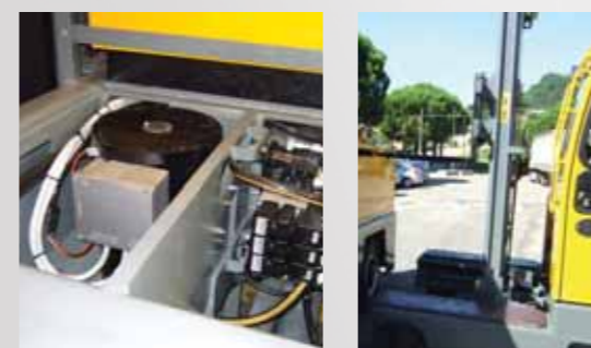
Some details of the 120 V technology fitted on the new BAUMANN electric sideloader EGX 50-70.
